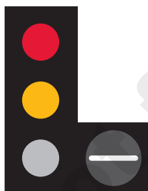
The signal mounted to the right gives instructions to tram drivers; these instructions may not be the same as those given to drivers of other vehicles
