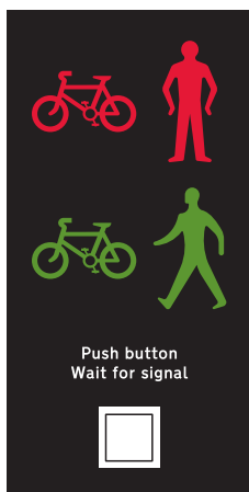
Near-side signals for toucan crossing
