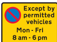
Repeater sign within a loading area
