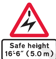
Electrified overhead cable and the safe height beneath it (usually associated with an overhead electrified railway or tramway). On the approach to a junction, the plate may include an arrow to indicate the direction of the level crossing
